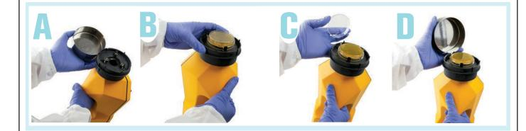
3. Gently place the closed plate into the TRIO.BAS clips. Remove the media plate lid and set on a clean surface with the inside of the lid facing down so that no particles settle into the lid.
